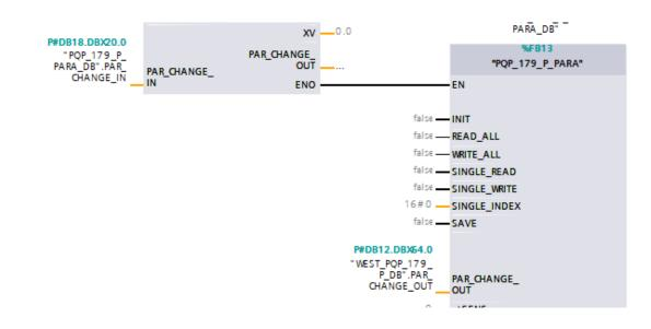
Due to the handling of the instance DB of the parameter module as an image of the setting values, it is not recommended to create it in the form of a multi-instance.
