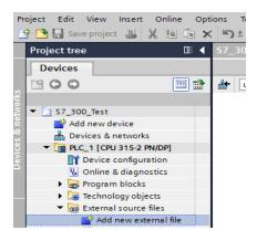
2.) Then click on the imported file with the right mouse button and select the option "Generate blocks from source". After the translation, the driver block is available in the block folder.
